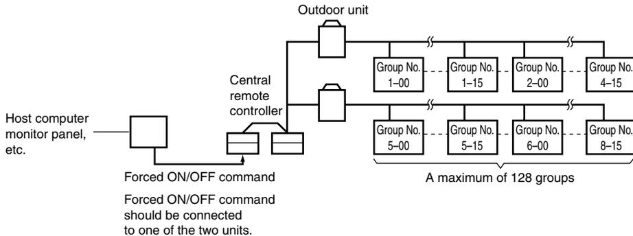
(The central remote controller and the separately sold remote control adapter circuit board or group remote control adapter cannot be used together.)
