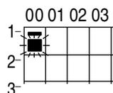
The display “” flashes under the group No. where the indoor unit that has stopped due to malfunction.
