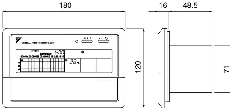
When using this unit an electric parts box of KJB311A is required.
