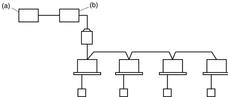
You can perform the normal operation, take off the malfunction contact point and unified start/stop by contact point, all by connecting this unit with the unification adaptor for computerized control. For further details, ask your DAIKIN dealer.
