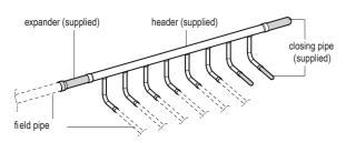
Use the supplied heat insulation material to insulate the headers against heat.
