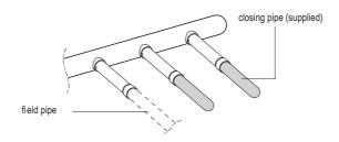
For connecting the field piping to the inlet of the liquid header:
