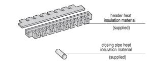
Apply the heat insulation material and seal all connections with tane.
