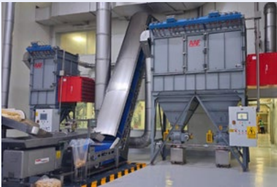
Dust collector installed at a food factory in Mexico
